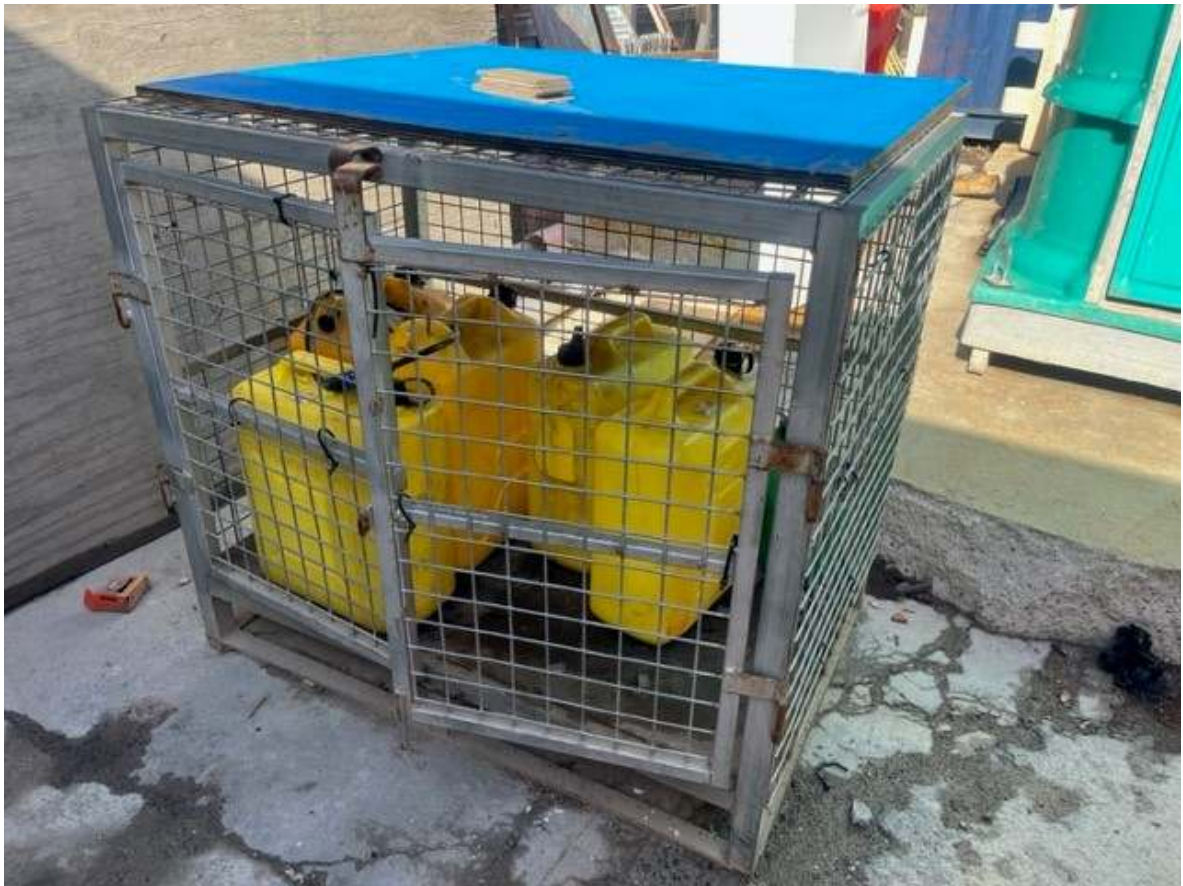
Photo 6: Diesel storage was non-compliant in the material storage area. Adequate bunding and Flammable liquid signage is required.
