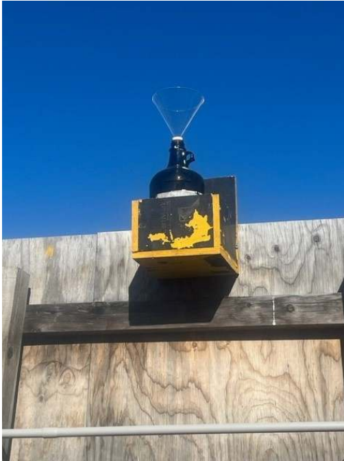
Photo 7: Dust deposition monitor in place
