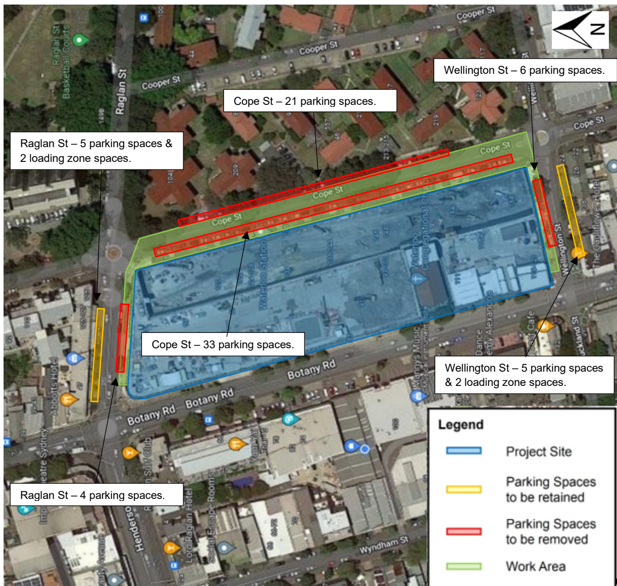
Figure 13: Affected Parking Spaces
