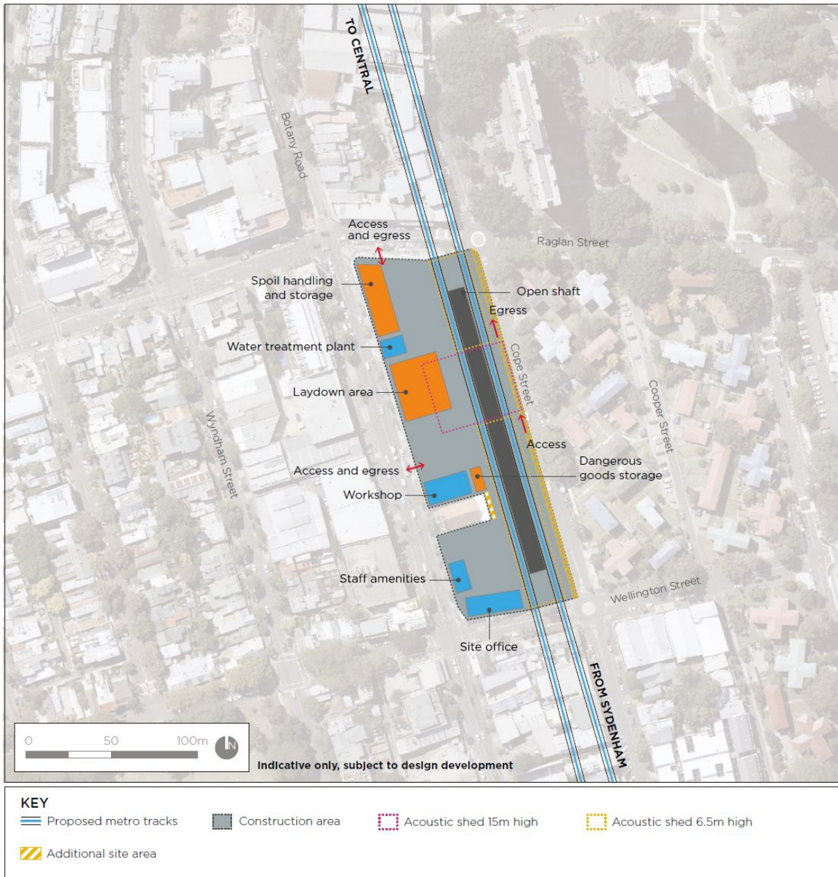
Figure 3-18 Revised Waterloo Station construction site – indicative location and layout
