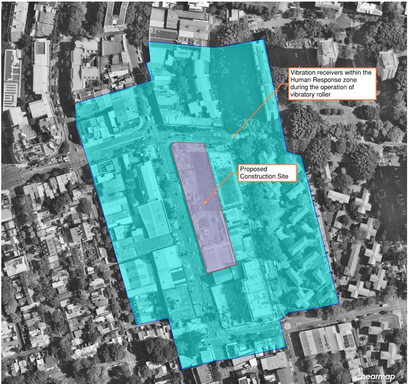
Figure 9 - Overview of the site and extent of the receivers closer than the Human Response zone for the operation of 10T Vibratory roller
