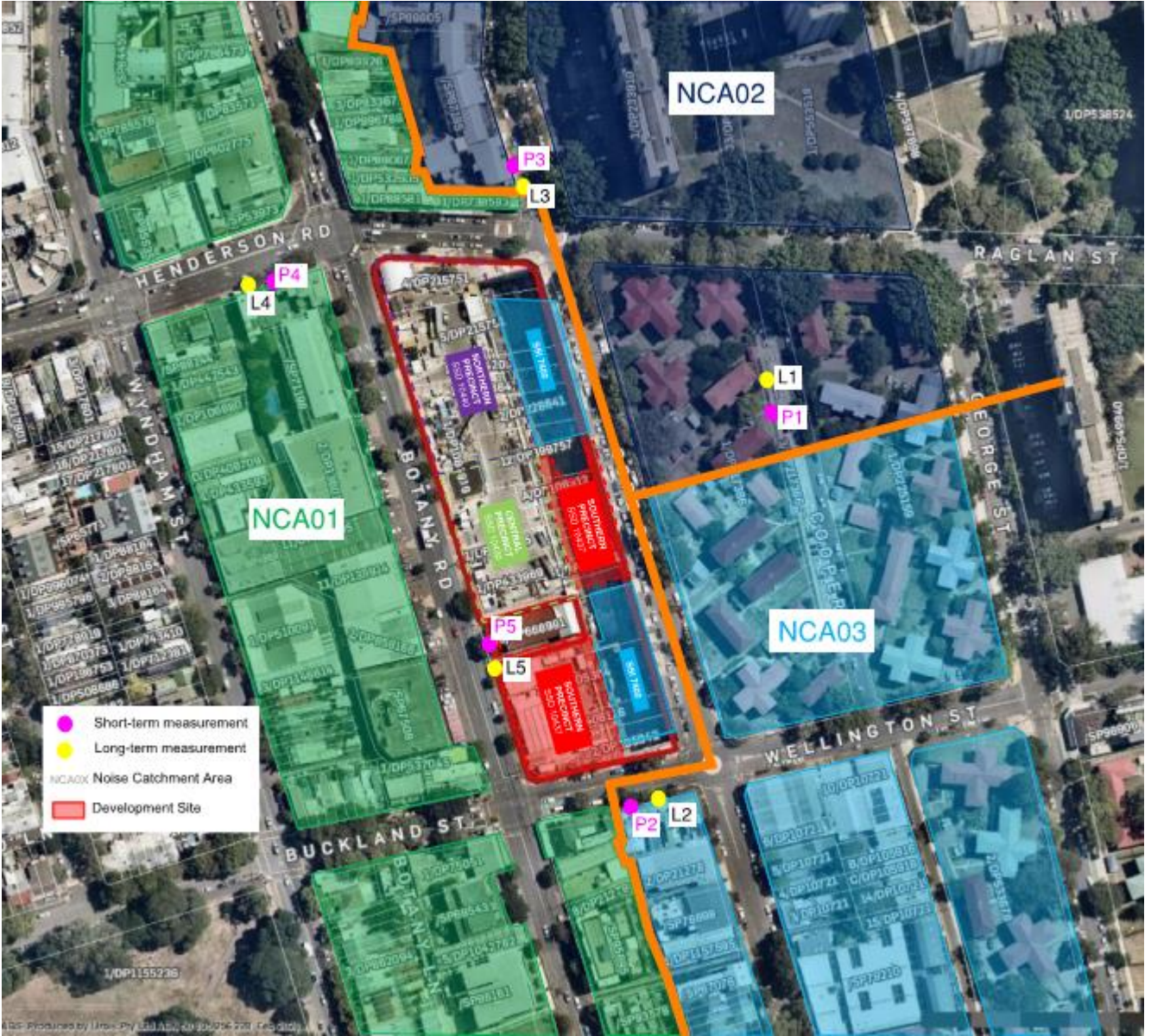
Figure 6 - Overview of the site, surrounding noise-sensitive receivers and measurement locations conducted by Stantec Australia
