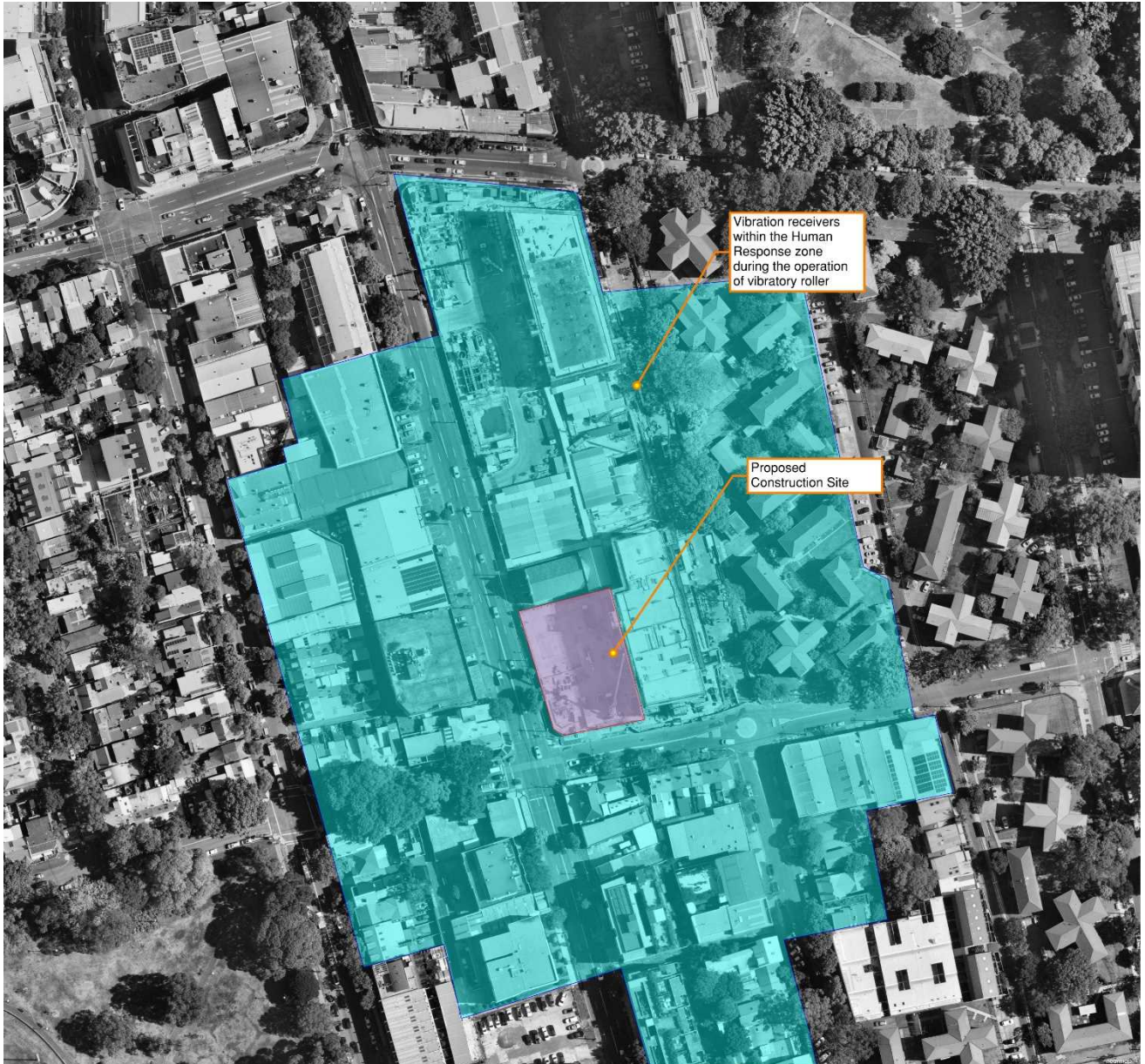
Figure 10 - Overview of the site and extent of the receivers closer than the Human Response zone for the operation of 10T Vibratory roller for the Southern Precinct Works
